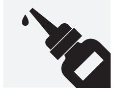
This method uses a liquid, known as thread locking adhesive, to prevent a bolted joint from loosening. The adhesive is applied to the thread of the fastener. Adhesives are not restricted by the size of the fastener used; however, they do pose a risk of chemical exposure and may be hazardous to health. They can also have a significant adverse effect upon the torque / load ratio, resulting in uncontrolled preload during tightening.
