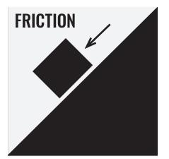
Friction locking methods are based on preventing surfaces from sliding against each other by increasing the resistance (friction) between these contact surfaces. Increased friction between the male and female threads, or between the fastener and contact surface, creates a resistance to loosening. Locking devices that use this principle include split ring, serrated and tooth washers. Nylon insert nuts fall into this category.
