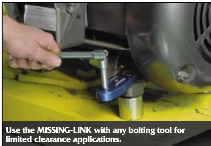
Missing Link working in tight location
