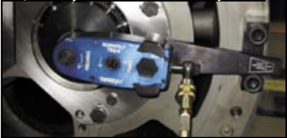
TBQ-6 with special reaction arm on compressor nut.
