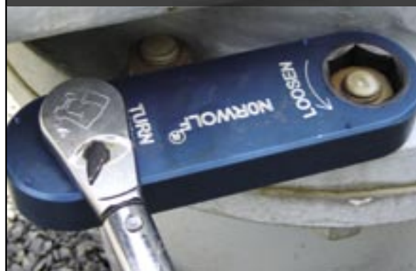
Missing Link working in tight location
