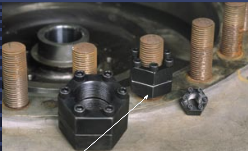
Threads on close to base reducing side load when removing stud.
