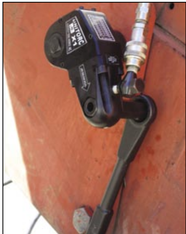
UNI-TORC using standard "knocker" wrench for added reaction length.
