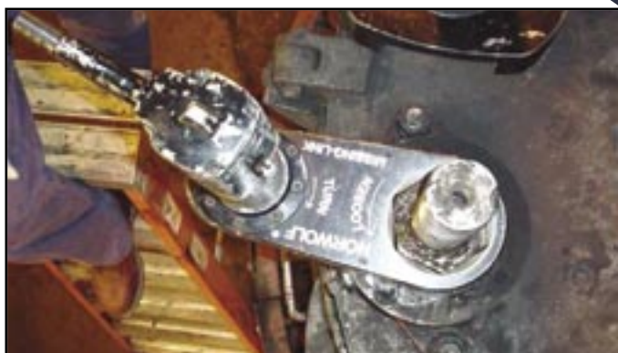
Norwolf Xcelink with Hub shown in use with an air multiplier on a coal pulverizer application.
