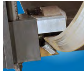
The I.D. tracker is ideal for end preps that require a consistent bevel on pipe with varying wall thickness.
