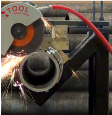
Concrete lined pipe can be cut cleanly. See the Video on our website showing this APS-438LRC with a 12" cut-off blade cutting this 8" concrete lined ductile iron pipe.
