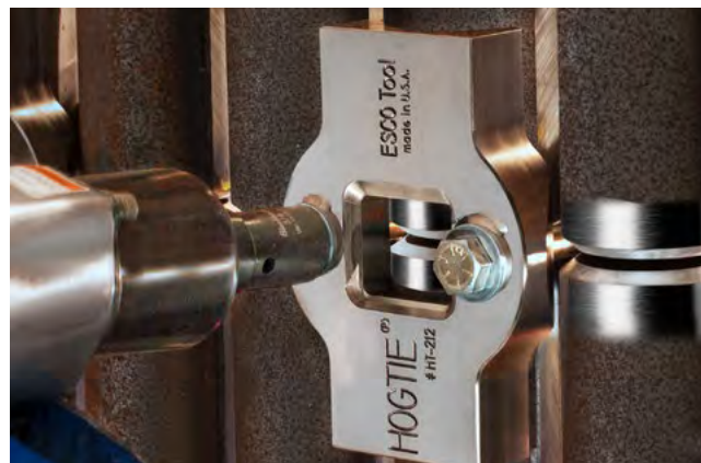
Available impact wrench draws the HOG TIE® assembly together for fast tube end alignment.
