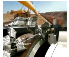
Compound bevels of 37.5° x 10° can be achieved with formed cutters.
