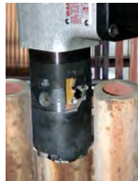
The ESCO patented membrane and overlay removal heads use round tapered inserts that can be rotated when worn and install and removed with a tap and a hammer.
