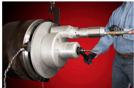
Compound bevel, face, and bore on 24" carbon steel pipe, 2" wall and wall variance of 1/4"
